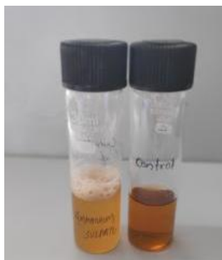
Figure 2. The media precipitated with ammonium sulphate and the control after 24 hrs of incubation.
